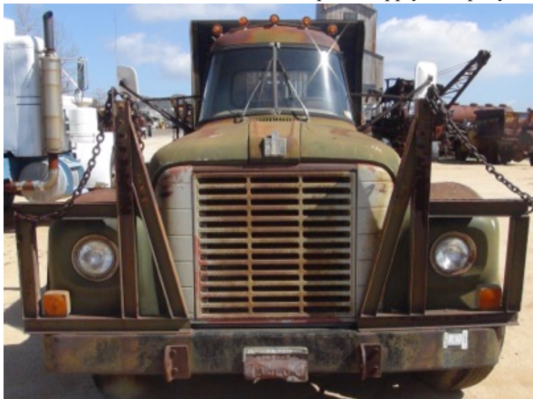
The 1964 International flatbed truck donated by Reliable Pipe & Supply Company. Notice the special cab with spaces on each side for loading long sections of pipe.
